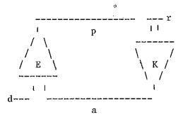
If a = K(r + p) and p = E(a + d), then we have a feedback situation. For this combination to be stable, the feedback must be negative, so K and E must have opposite signs. That is not, however, the asymmetry of which I speak, as either one can be negative. To see the asymmetry, we must solve the system equations as a simultaneous pair, to get
